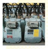
The meters are then read periodically and the ERTs checked for accuracy, providing a near real-world indication of how they will perform over time. Some of these ERT Modules have been part of these tests since 1991. If an inaccuracy or failure is detected, technicians immediately investigate the cause of the inaccuracy or failure.
