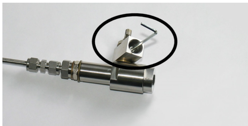
Figure 16 Removing the Leak Screw
