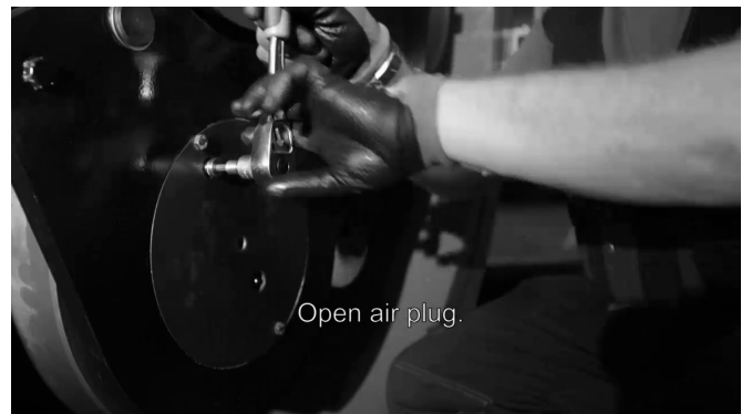
Figure 21. Opening the air plug
