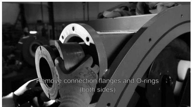
Figure 15. Removing the connection flanges and O-rings
