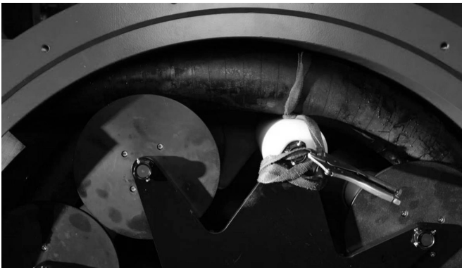
Figure 17. Securing the guide roller 2
