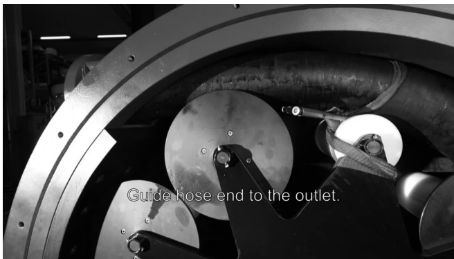
Figure 28. Installing the hose 6
