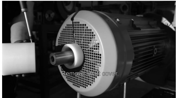
Figure 6. Removing the motor shaft cover
