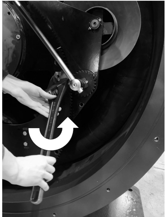
Figure 11. Removing the compression key
