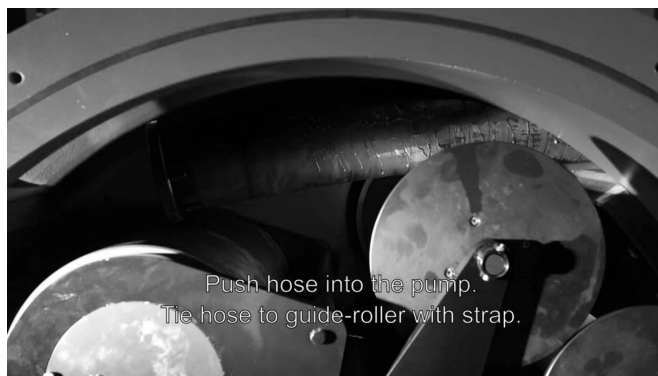
Figure 25. Installing the hose 3
