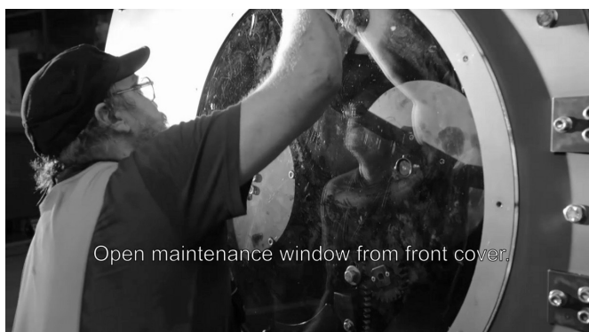
Figure 41. Opening the maintenance window
