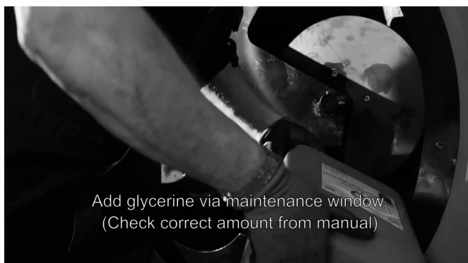
Figure 42. Adding glycerine to the pump
