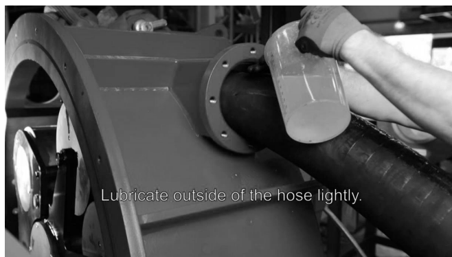
Figure 24. Installing the hose 2
