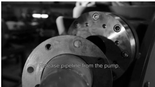
Figure 4. Removing the hose
