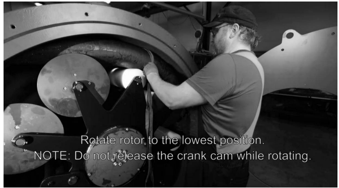
Figure 35. Installing the hose 13
