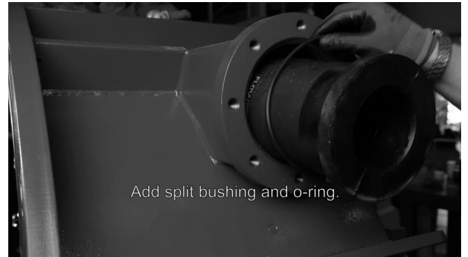
Figure 29. Installing the hose 7
