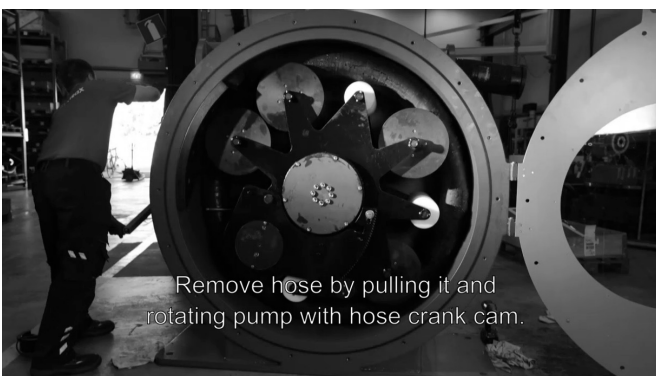
Figure 18. Removing the hose
