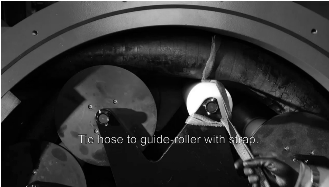
Figure 16. Securing the guide roller 1
