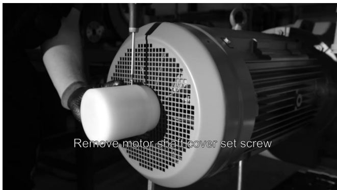
Figure 5. Removing the motor shaft cover set screw
