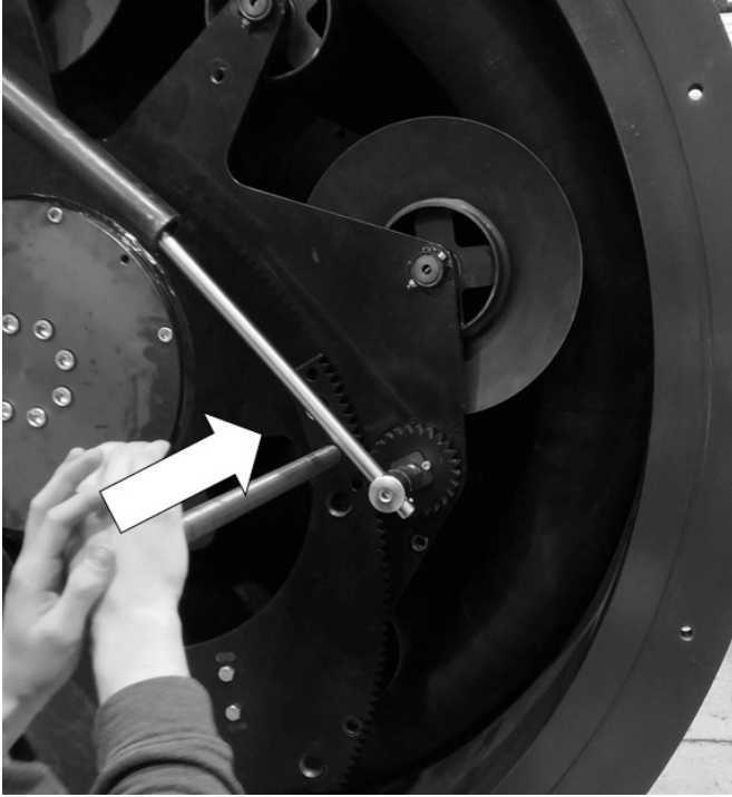
Figure 37. Installing the hose 15
