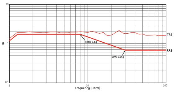
Lowest equipment natural frequency: 8.4 Hz Qualified by shake-table testing, Wyle Laboratories, Dec. 2005
