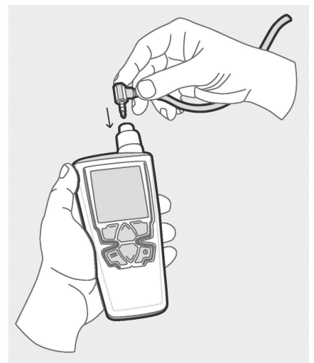
Snapping a connector to the indicator HM40 to read the measurement results.
