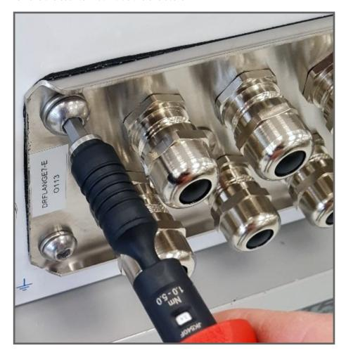
2. Push the screws back to place and insert the serrated lock washers on the screws.
