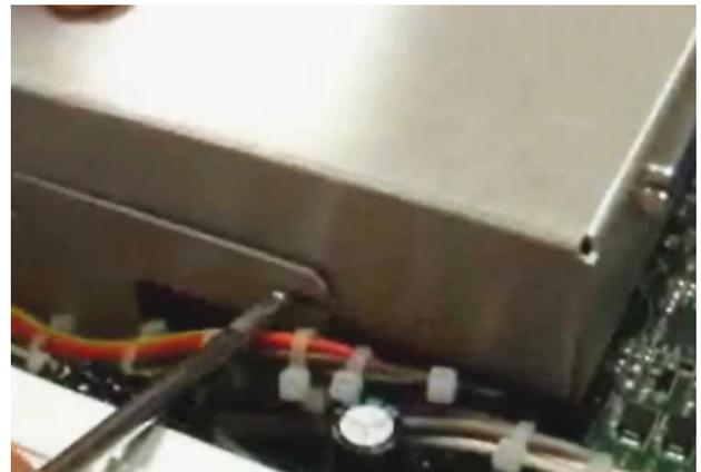
9. Mount front cover of the control module that was dismantled in Step 3. Fasten 4 screws holding it.
