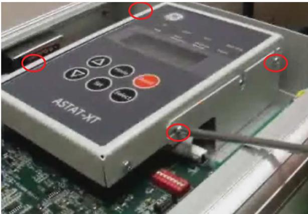
5. Disconnect flat cables from display unit and from main PCB SMDP2000.
