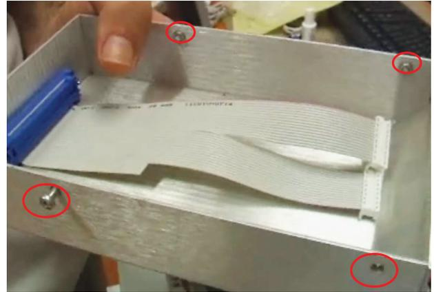
7. Connect 2 flat cables from dummy cover to main PCB SMDP2000.
