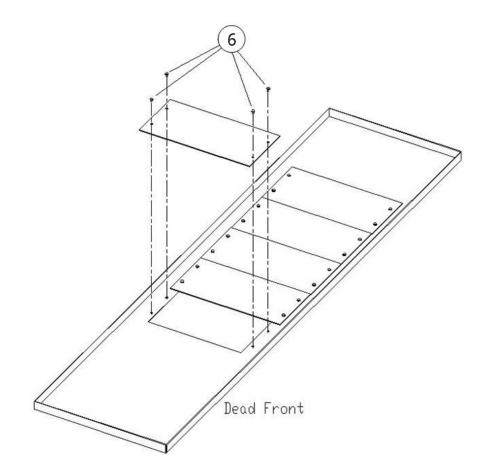
Figure 2. Removing the shield inserts from the shield for THQB breaker installation in A-Series<sup>®</sup> II Panelboards.
