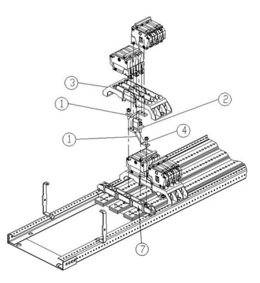
*Figure 1. Installation of a THQB circuit breaker kit on interior, catalog number ASPP6QB12D, into an A-Series*<sup>®</sup> *II Panelboards.*
