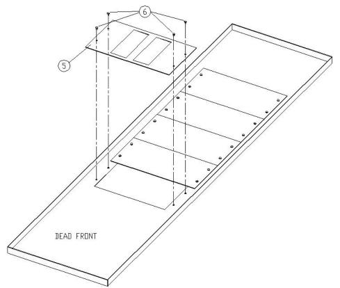
Figure 3. Attaching the shield insert to the shield for THQB breaker installation in A-Series<sup>®</sup> II Panelboards.
