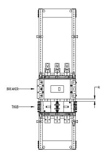
Figure 4. Distance between breakers
