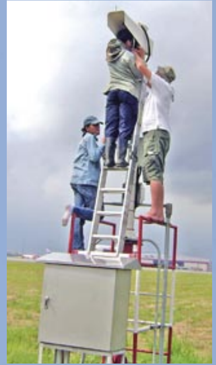
Vaisala’s transmissometers provide accurate data for Runway Visual Range (RVR) assessment at the Second Bangkok International Airport.
