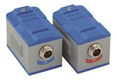
Temperature Range – 30...+90°C Max Cable length: 200mt TTS-100-TS2-NG Range: DN15...100 Working Frequency 1.5 MHz TTS-100-TM1-NG Range: DN50...1000 Working Frequency 1 MHz TTS-100-TL1-NG Range: DN300...6000 Working Frequency 0.6 MHz
