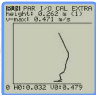
Flow profile directly indicated on the display.
