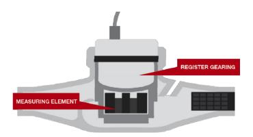
Water meter registers typically are one of three types: direct read, pulse-based (pulser) and absolute encoder. Direct read meters have a display that must be read by a utility meter reader. Absolute encoder registers are read using an inductive probe or by a serial communication-based AMR/AMI device. Pulse-type registers generate an electronic pulse that is counted by the AMR/AMI device.
