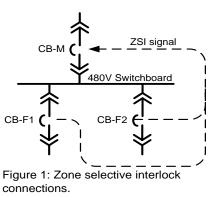
4. Any time the feeder circuit breaker picks up on short time and ground fault, it will send a restraint signal to the main circuit breaker.
