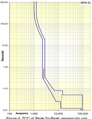
Figure 4: TCC of 'Peak-To-Peak' sensing trip unit
