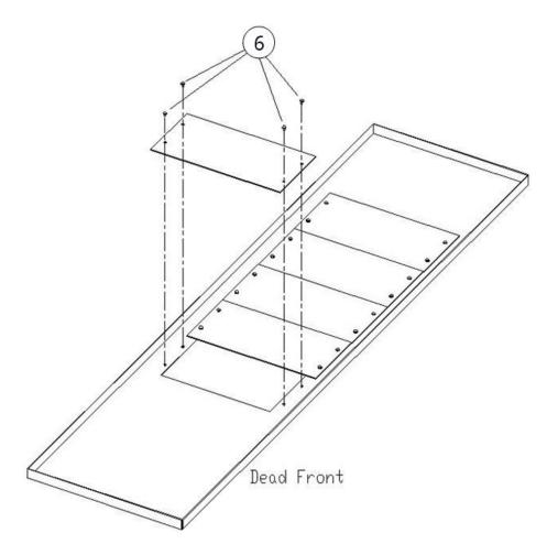
Figure 2. Removing the shield inserts from the shield for TEY breaker installation in A –Series $^{\text{@}}$  II Panelboards.
