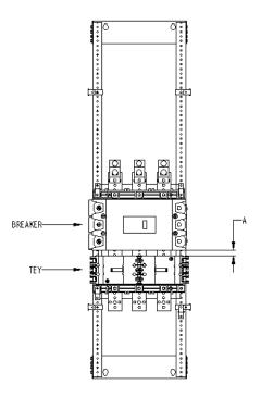
Figure 4. Distance between breakers
