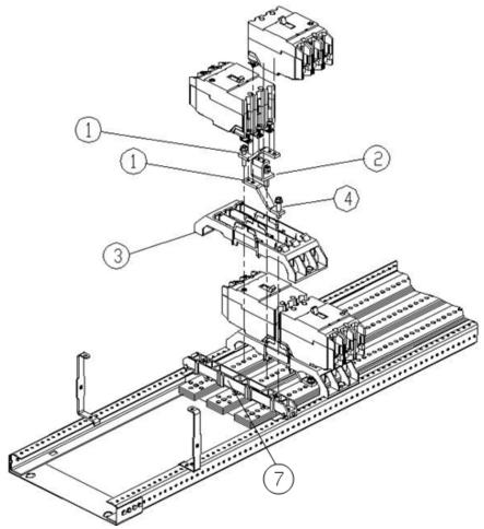
Figure 1. Installation of a TEY circuit breaker kit on left side of interior, catalog number ASPP6EY12D, into an A-Series® II Panelboards.
