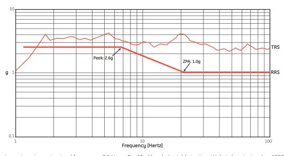
Lowest equipment natural frequency: 7.0 Hz Qualified by shake-table testing, Wyle Laboratories, Apr. 1998
