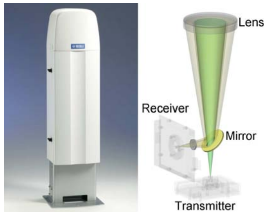
Figure 1: Vaisala Ceilometer CL31 and its single lens optical concept.
