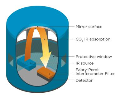
Structure of the CARBOCAP® sensor.
