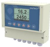
The 7300w² Monitor is the core to the WaterWatch² product range, the monitor is designed to interface with all the sensors in the WaterWatch² range. The monitor specification provides all the connections required for 1 or 2 sensors, systems can be expanded by the use of expansion boxes to include multiple sensors. The maximum number of sensors will be limited by the practicalities of most sites. We anticipate 8 being a sensible maximum although many more can be accommodated.
