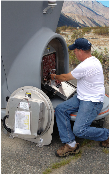
Field service technician removing current array and replacing it with the upgrade.
