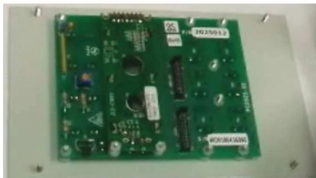
8. Mount the dummy cover (Item C) to soft starter frame and fasten with 4 nuts.
