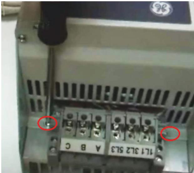
7. Dismantle 4 nuts holding front cover to soft starter frame.
