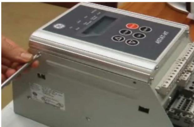
6. Remove the front cover and disconnect flat cable connections from main SMDP2000 and from keypad PCB2025.
