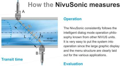
The NivuSonic measurement principle is based on detecting the transit time of ultrasonic signals between two sensors (A and B). The transit time in flow direction t, is shorter than it is against the flow direction t<sub>2</sub>. The difference between both transit times is proportional to the average flow velocity along the measurement path v<sub>m</sub>.
