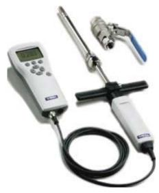
Vaisala HUMICAP® Hand-held Moisture Meter MM70
