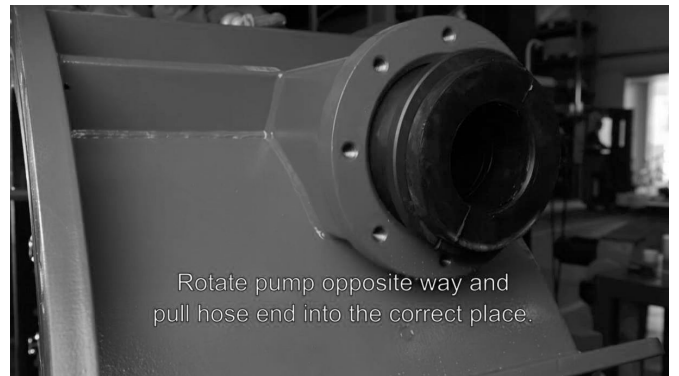
Figure 30. Installing the hose 8
