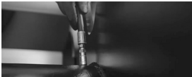
Figure 22. Adding grease to the rotor bearings
