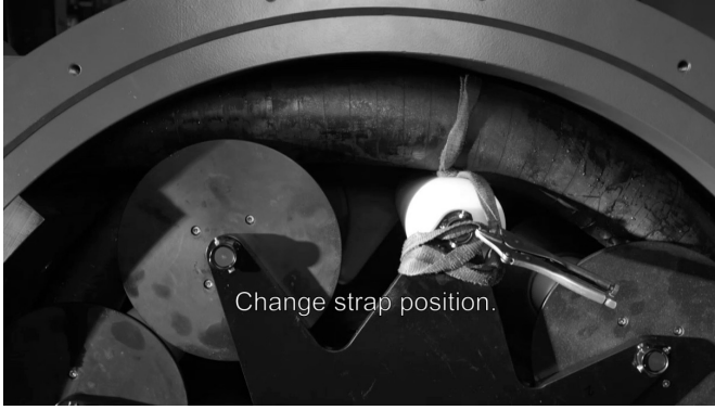
Figure 32. Installing the hose 10
