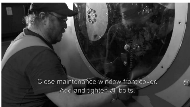
Figure 43. Closing the maintenance window
