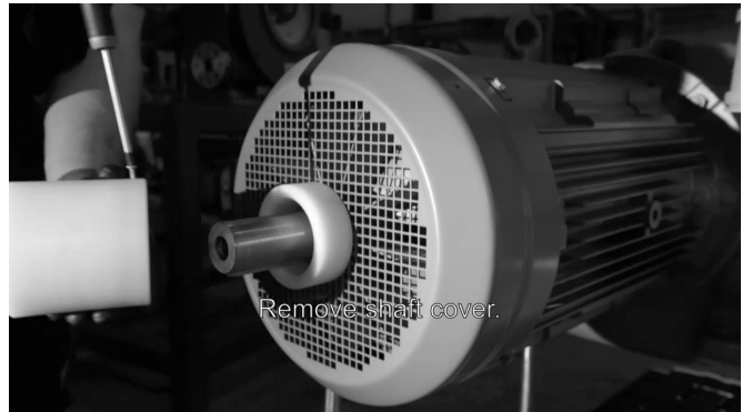
Figure 6. Removing the motor shaft cover
