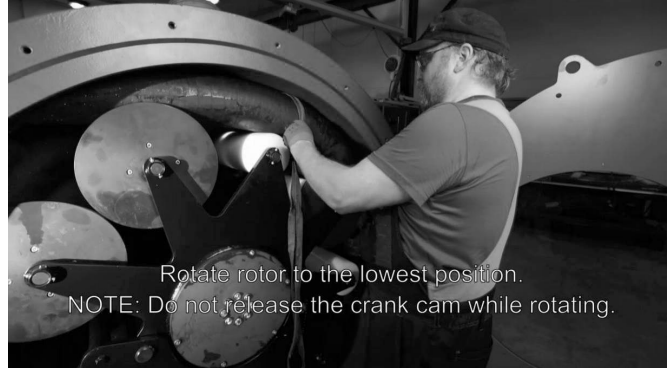
Figure 35. Installing the hose 13
