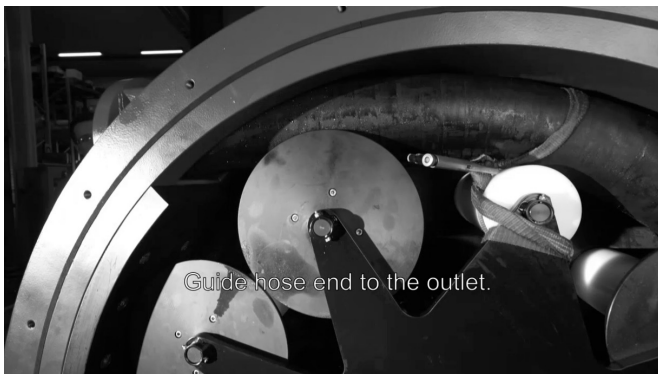
Figure 28. Installing the hose 6
