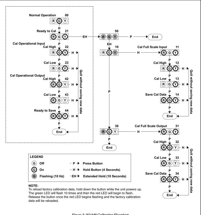
Figure 3: WV448 Calibration Flowchart
